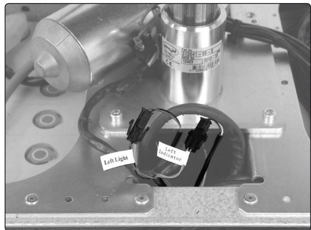
Fig. 3. The connectors on the front lights cabling are positioned next to the seat lift/seat post.
