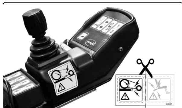
Picture 3. Sticker to be applied on the control panel
