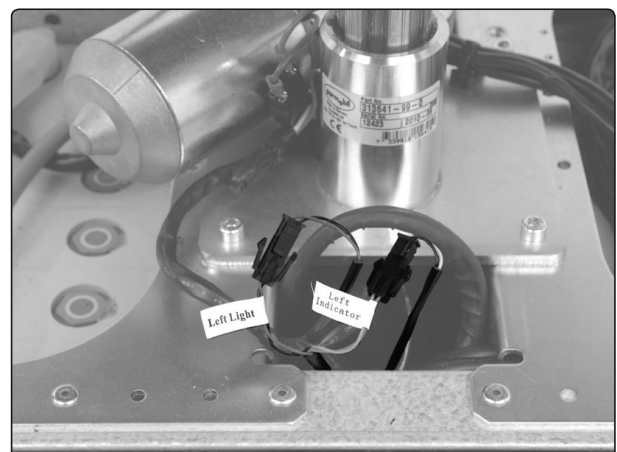
Fig. 3. The connectors on the front light and indicators cabling.
