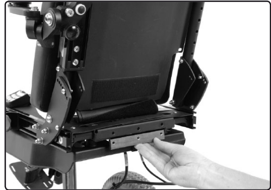
Fig. 2. The bracket is fitted on the inner side of the seats rear edge.
