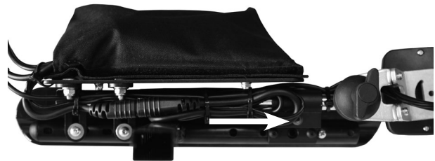
Fig. 19. The control panel holder is fixed with a screw.
