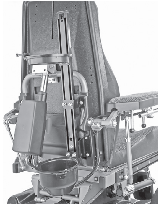
Fig. 5. The mounted accessory. Three existing screwholes on the back joint are used.
