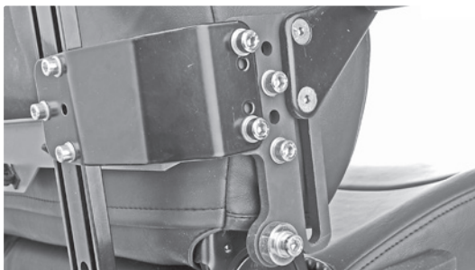
Fig. 8. The accessory mounted on the reinforcement.
