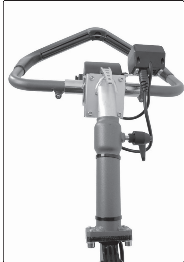
Fig. 3. Cabling secured with cable ties.
