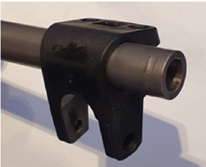
Fig.2 Slide the Clamp rear axle lower, pos.2, on each side of the rear axle, pos.1 (Fig 1)
