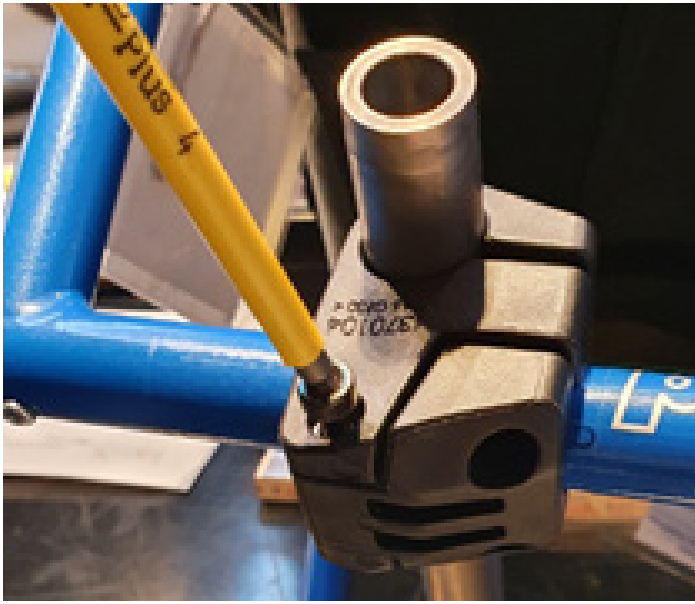
Fig.3 Now mount Clamp upper, pos.3 together with Bolt M5x35, pos.4 so that the Clamps, pos.2 and 3 is together (Fig 1)
