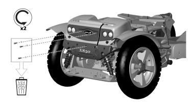
11 Turn the distance screws clockwise (torque 9.8 Nm) into the holes in the top cover.
