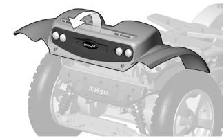
**3** Disconnect the light cable from the electronics and release the cable from the cable holder.
