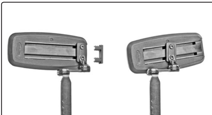
Fig. 7. Assembly of cushion and bracket. Left. If the cushion has a plastic plug, remove it. Then slide the nuts into the grooves on the cushion. Right. Fix the cushion in the desired position by tightening the screws. Remount any plastic plugs.
