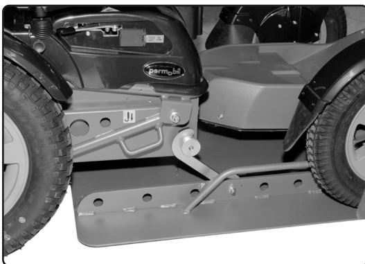
Fig. 6. Locking of chassis by rear hook.
