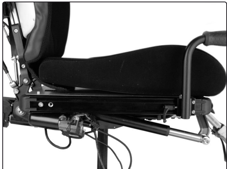
Fig. 3. The raising handle mounted on Corpus 3G.
