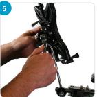
Slide the Mounting Bracket post into the upper post clamp and tighten with a 13 mm wrench.
