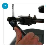
Once the tablet is positioned properly, securely tighten all panel mount screws and post clamps nuts. This is critical to ensure the security of the tablet and its desired position.
