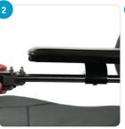
Slide Swing-Away Mount post into Panel Mount and tighten clamp screw with a 5 mm Allen wrench.
