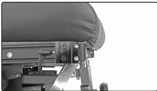
Fig. 5. The bracket mounted as far forward as the fully inserted plastic plug will allow.
