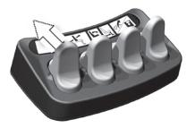
49 When the LED:s flash red the system is requesting a restart. The system may require multiple restarts. Power the chair off and back on again. The switchbox will return to normal operation.
