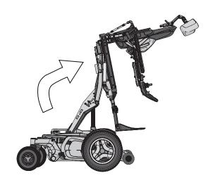
19 Remove the bracket holding the end of the actuator and scrap it. The bracket can look different depending on the revision. See A, B or C.
