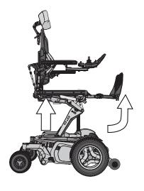
Remove the seat cushions by lifting it straight up. It is attached by means of velcro on the rear of the cushion. Remove the seat plates, which are held in place by four screws.
