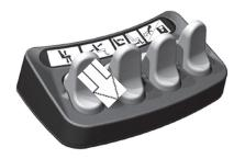
19 The goal is to anterior tilt the seating to a position that allows easy access to the underside of the top plate. After reaching this position power down the chair.
