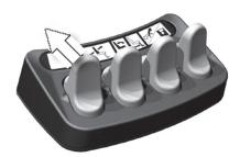
When the LED:s flash red the system is requesting a restart. The system may require multiple restarts. Power the chair off and back on again. The switchbox will return to normal operation.
