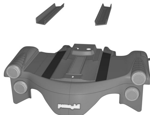
Fig. 5. Peel off the protective tape and mount the crush protection at the markings on the chassis cover.
