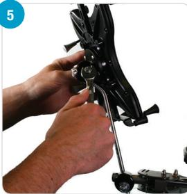
Slide the Mounting Bracket post into the upper post clamp and tighten with a 13 mm wrench.
