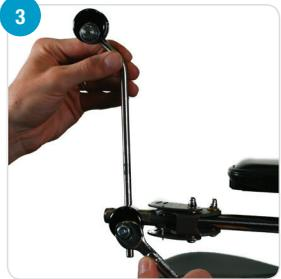
Orient the upper arm vertically and tighten with 13 mm wrench. Position the clamp far enough forward to avoid interfering with the swing-away mechanism. The clamp lock nuts should face outward for better access and positioning.
