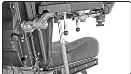
Fig. 14. Fix the cable in the back joint's protective cover.
