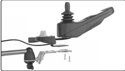
Fig. 11. The button box is attached under the joystick.
