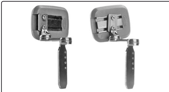
Fig. 7. Assembly of cushion and bracket. Left, the bracket nuts are slid into the cushion grooves. Right, the cushion is fixed in the desired position.
