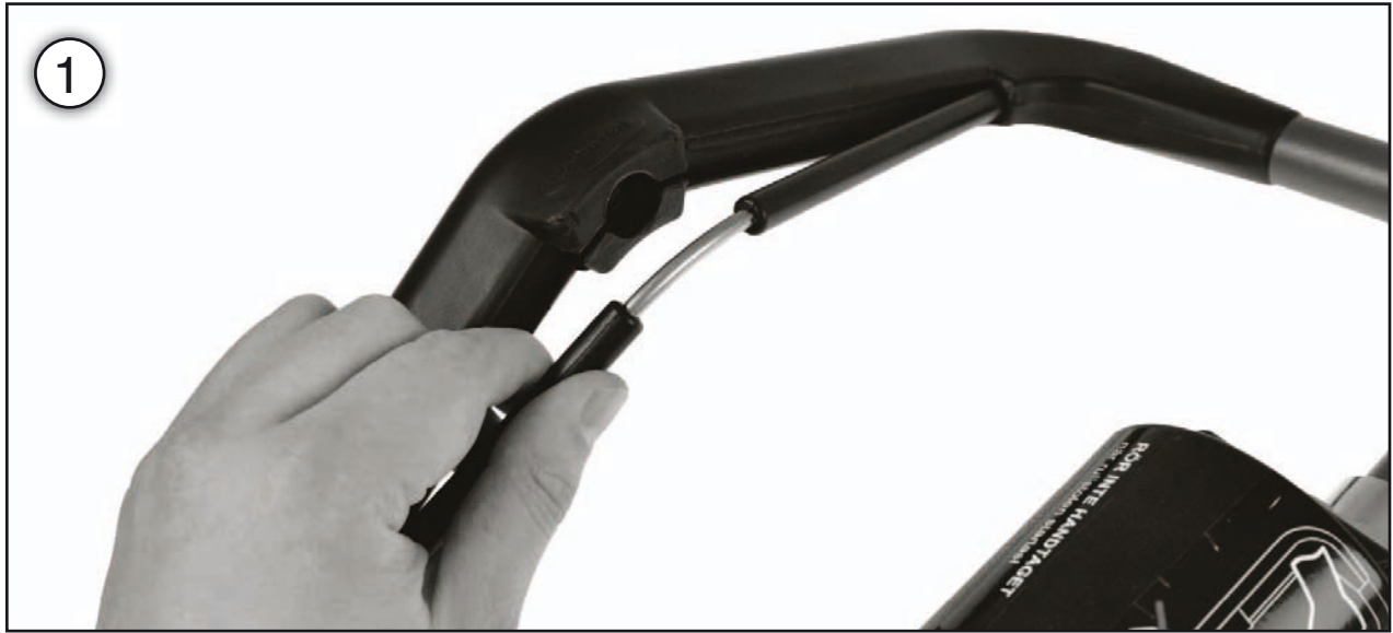
Figure 1. Press your fingers underneath the safety grip and pull to get the rod loose from the holder in the rubber handle.
