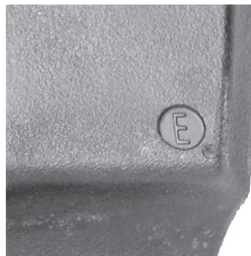
Fig. 8. The moulded identification letter.
