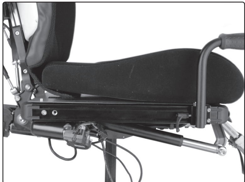
Fig. 3. The raising handle mounted on Corpus 3G.
